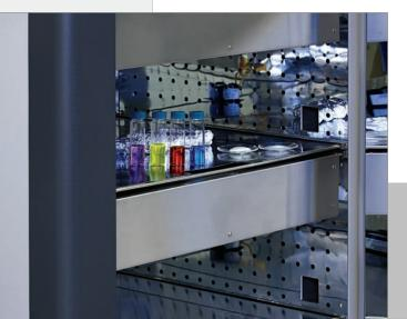
We meet the requirements of these various testing scenarios and ensure compliance with each protocol by constant monitoring of temperature and light exposure. We also test container integrity with our photostability chamber, as well as examine potential light degradation compounds in conjunction with method validation studies.
